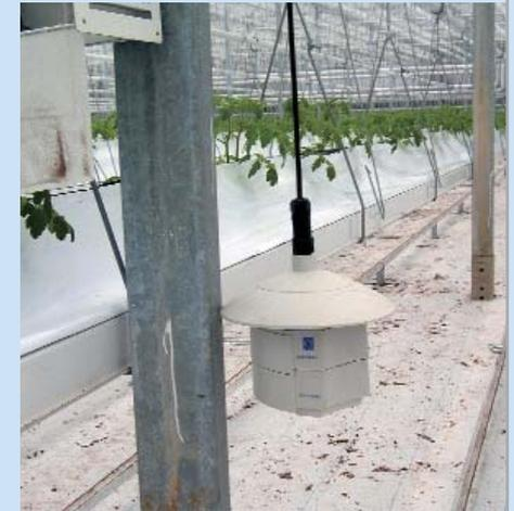
(pictured) that can now be integrated into its all electronic measuring boxes. The cost of maintenance and calibration is said to be a fraction of the cost of more traditional systems that use sampling tubes and pumps.
