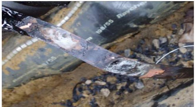
Reinforcing tape failure results in the lead sheath being unable to contain the oil pressure, leading to 'bulging' of the sheath and, eventually, oil leaking from the cable causing environmental and reliability performance issues.
