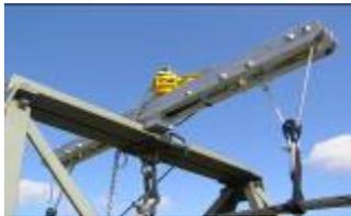
**Earthwire Lifting Beam** – This project is developing a lightweight lifting beam for suspension tower peaks to provide a lifting point for the replacement of earthwire suspension fittings. An initial design has been manufactured and tested. Extensive trials successfully completed. A possible improvement to the design and a reduction in weight is currently being investigated.
