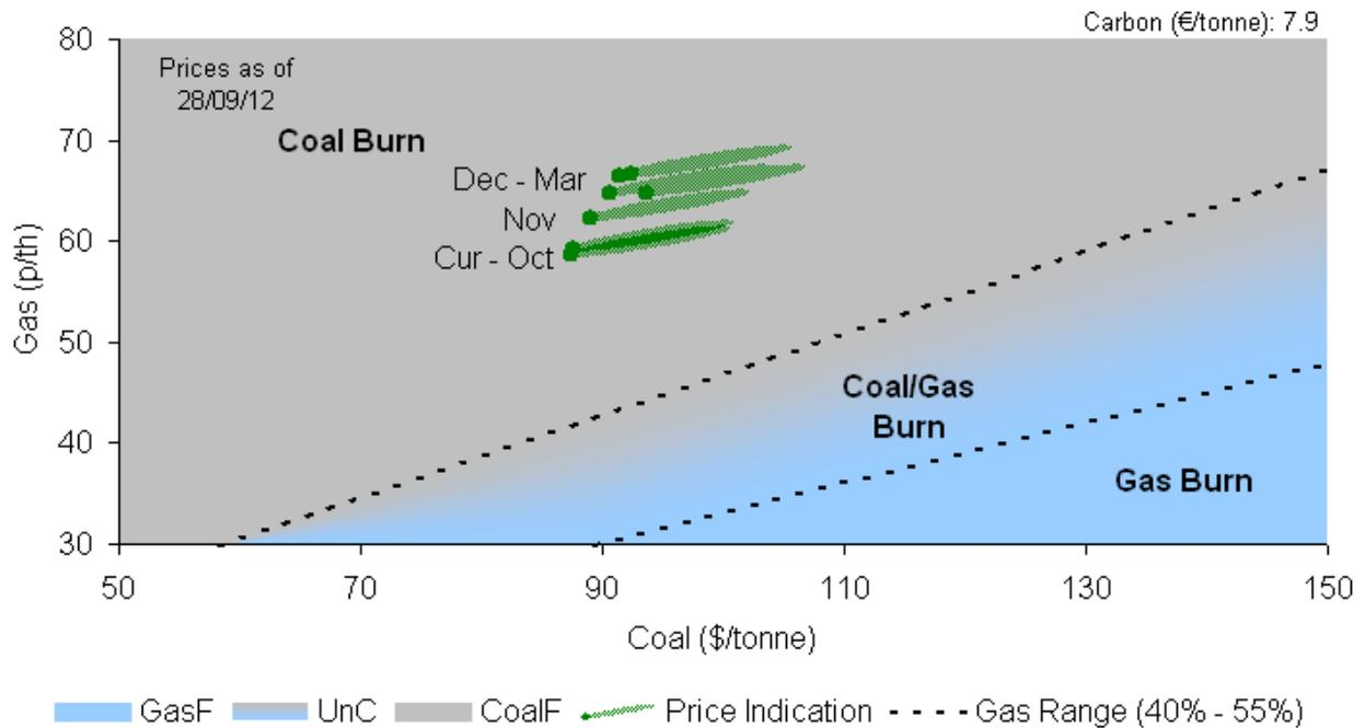
17. The chart shows how the forward prices for winter 2012/13 strongly favour coal burn over gas. For gas and coal to be equitable the gas price for winter 2012/13 needs to fall by about 40% or around 30p/therm, alternatively there needs to be a further increase in the coal price by about \$80/tonne.
