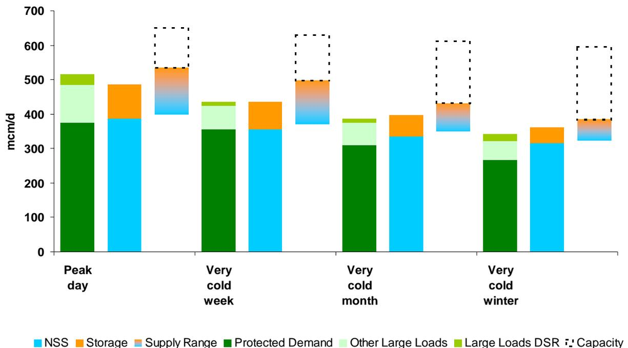
114. Apart from a 30 mcm/d requirement for either additional NSS or storage or an equivalent demand side response for a peak day, all demand could be met by the central case supply assumptions for all demand conditions evaluated. The wide range of the NSS and storage at peak and the potential for a modest demand side response indicates that a requirement for 30 mcm/d should in principle, be achievable.
