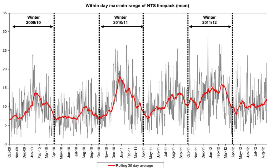
137. Large linepack reductions are caused when the demand from the network, exceeds the rate of supply entering the network. This usually occurs at the start of the gas day often as power demand increases (see **Figure G24**), supplies then tend to increase later on in the day, and as long as the rate of supplies is above demand, linepack recovers.
