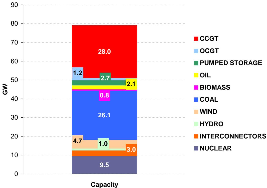
186. The net reduction is due to a combination of gains and losses. Capacity has reduced due to the closure of the two oil fired units at Grain and the extension of the ongoing repairs at Shoreham but capacity has increased due to the commissioning of the last two units at Pembroke and more wind farm capacity coming on the system.
