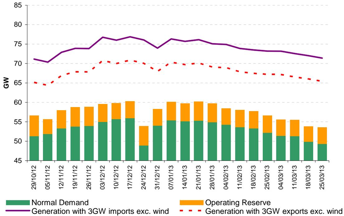
211. **Figure E6** shows Normal Demand and the declared generation availability excluding wind. This shows that there is adequate margin without wind generation available under optimum declared availability, although the minimum surplus on this basis drops to 13%, assuming the interconnectors are at float.
