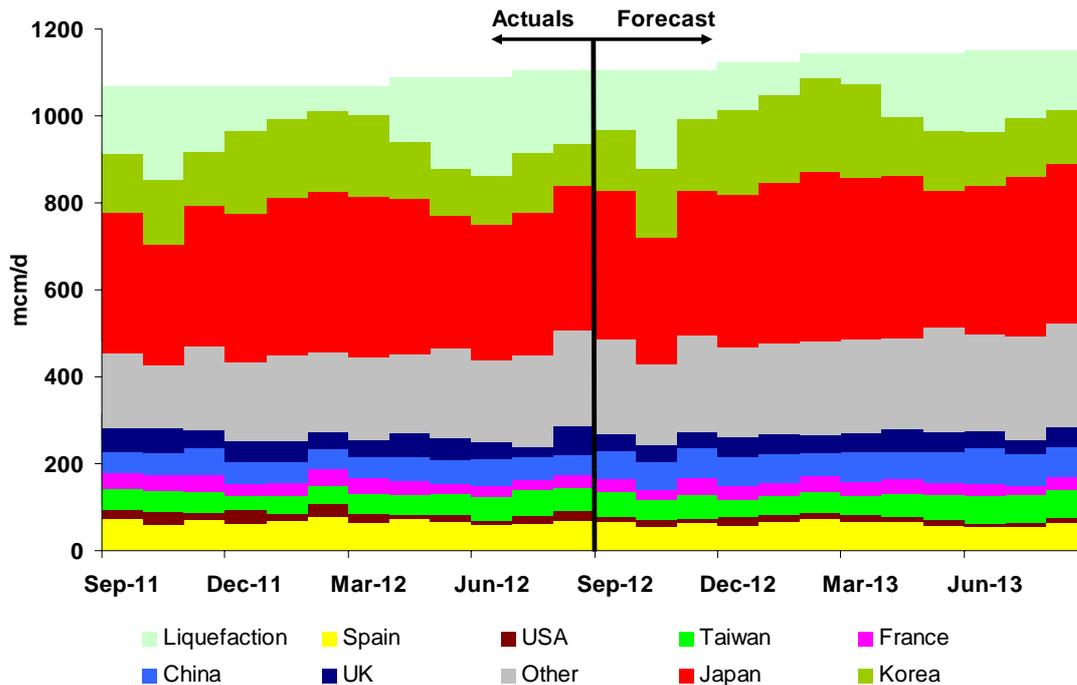
73. The chart shows an increase in LNG liquefaction capacity since last winter, with Australia's Pluto facility starting up last spring. The Angola project is expected before the end of 2012, while any new production in Algeria (Skikda / Arzew) may replace existing volumes rather than adding extra capacity.
