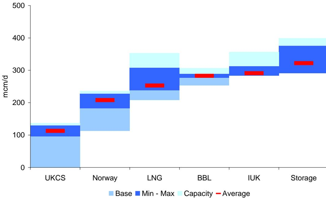
96. **Figure G17** shows an assessment of the supplies for when demand exceeds 400 mcm/d as a supply stack. Each supply source is stacked at the level of the '400 mcm/d' position. Theoretically each stack could commence at higher or lower positions to enable higher demands to be met.
