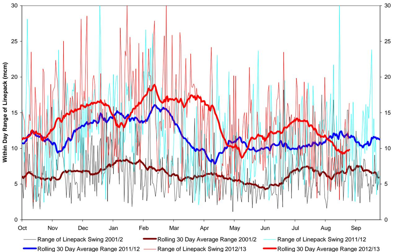
116. **Figure G22** shows both the daily range and the 30 day average linepack swing seen on the NTS in 2001/02, 2011/12 and for 2012/13 and suggests that this linepack swing has increased by 200% from the position of 10 years ago and by between 10 – 20% from last year.
