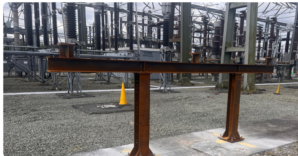
Long-term testing of weathering steel is underway at Deeside Centre for Innovation
