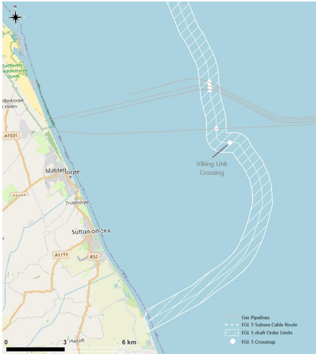
Plate 17.B.2 Location of EGL 5 subsea cable and pipeline crossings modelled. (OpenStreetMap used for basemap). The route for Viking Link was not available as a shape file and is therefore not shown on the plot. The southern most EGL5 crossing is where it crosses Viking Link.
