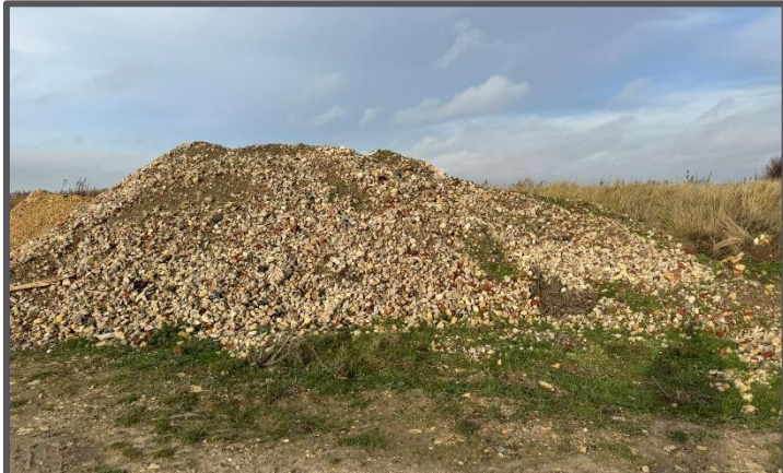
3a: View looking northwest of Stockpile 1, demolition waste (bricks concrete etc.).
