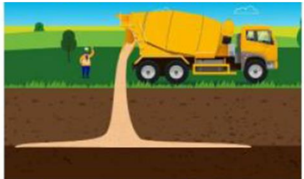
Step 4 Ducts are installed into the trenches; the trenches are filled with a mixture of sand and cement to manage any heat transmitted from the cables and then backfilled
