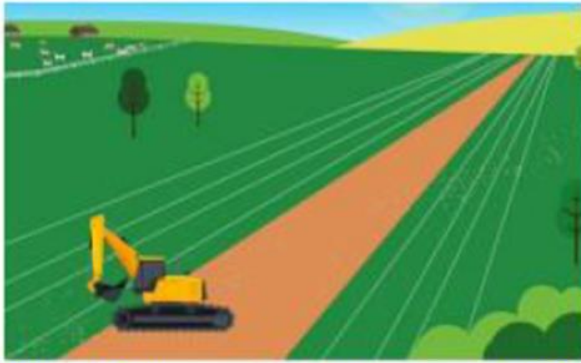
Step 1 Cables are installed in one (HVDC) or two (HVAC) trench(es), adjacent to the temporary haul route
