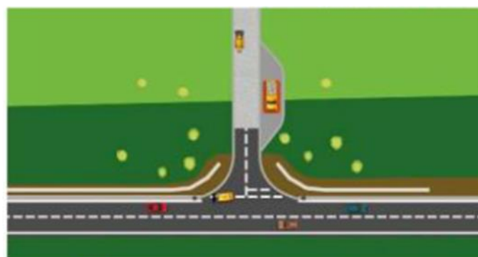
Step 5 Wheel washes are installed to reduce dust and soil leaving site
