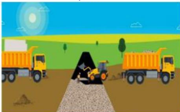
Step 3 Highways specification stone is then laid for the haul route surface
