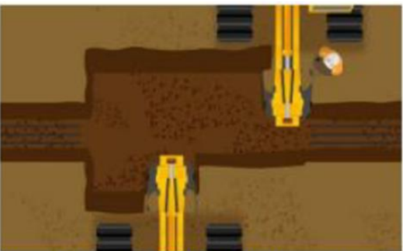
Step 5 Trenches are joined via a wider area called a joint bay
