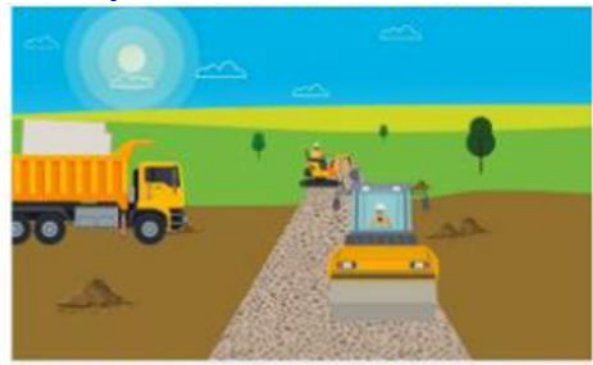
Step 4 The haul route is then rolled and topped with a layer of smaller stones which vehicles can drive over
