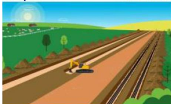
Step 7 The stored subsoil and topsoil are carefully replaced on top of the trenches and the haul roads removed. The land is reinstated and managed back to its previous condition
