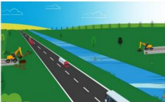
Step 1 The topsoil is carefully removed and stored for the temporary haul route and two pits are dug either side of the section of cable
