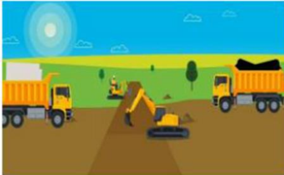
Step 1 The topsoil is carefully stripped from the land where the haul route would be built and stored whilst works take place
