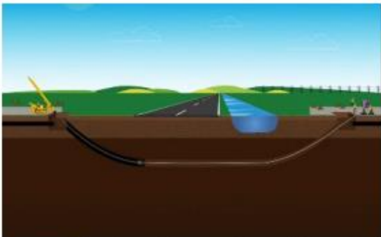
Step 4 The bond is used to pull the ducts (the tubes that house the cables) through the newly drilled route
