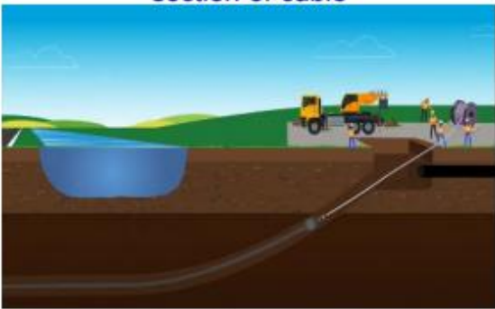
Step 3 A wire called a bond is attached to the drill and is pulled back to the other side of the works
