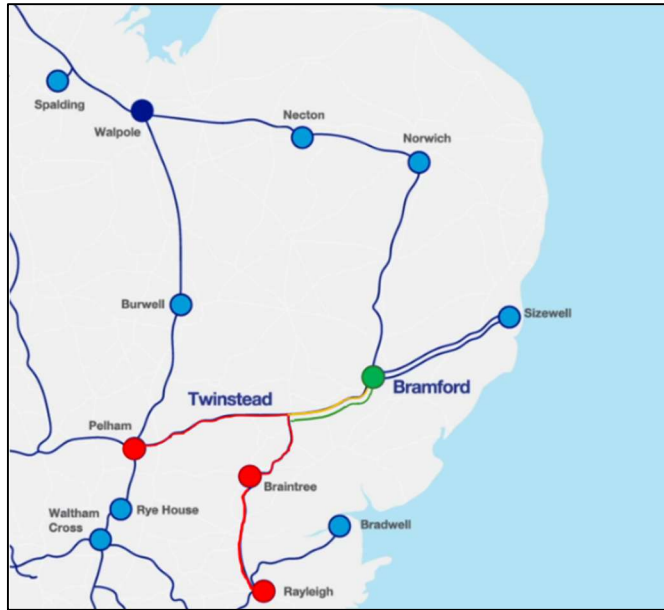
Figure 1: Key OHL sections to be upgraded by the Project and associated substations in red.
