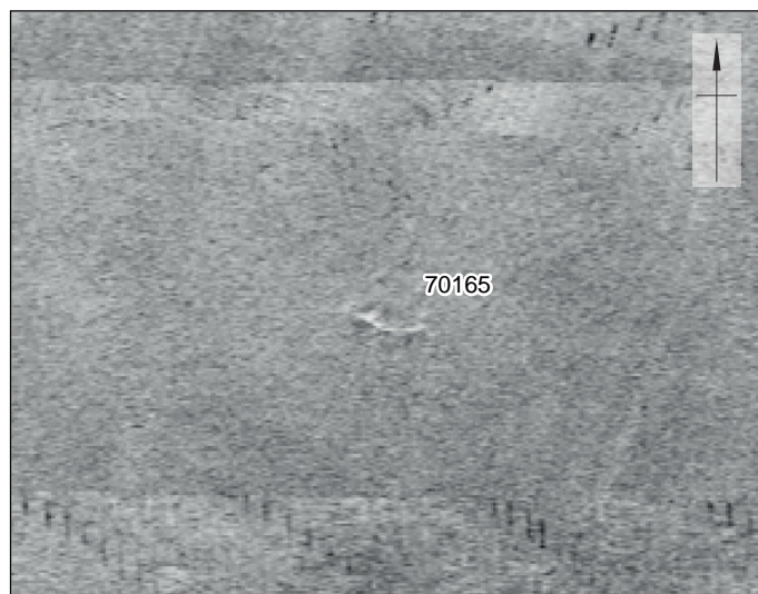
SSS mosaic image showing bright reflector anomaly 70165 , measuring 6.9 x 0.7 m
