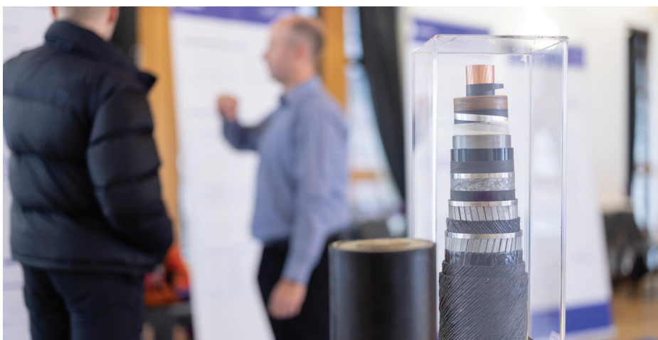
Cross-section of underground cable
