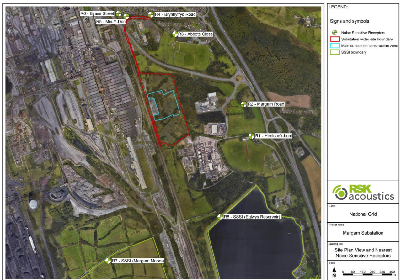
Figure 2.1 Plan view of Margam substation and nearby noise sensitive receptors
