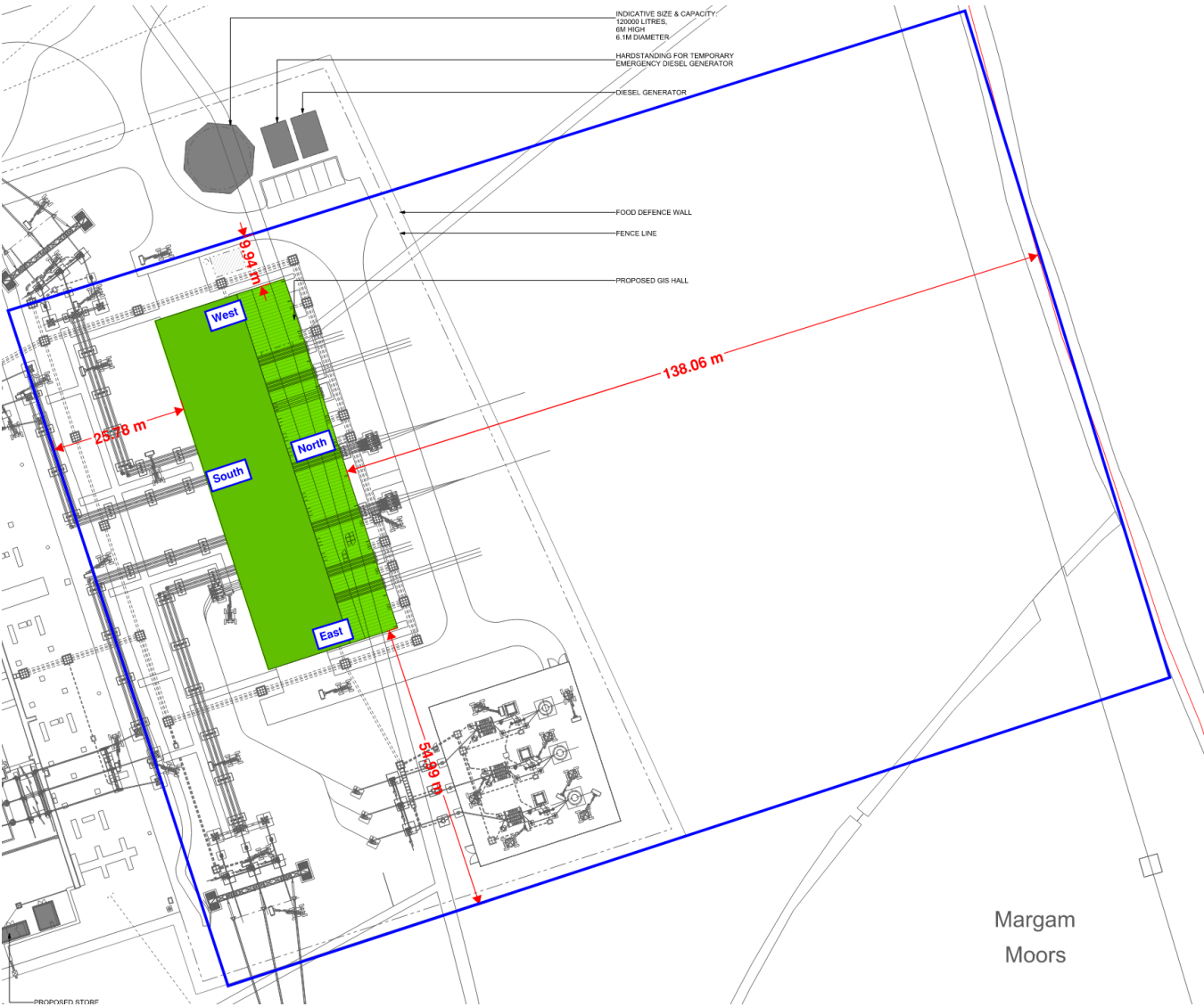
Figure 12 Relevant boundary distances for the Margam GIS Hall
