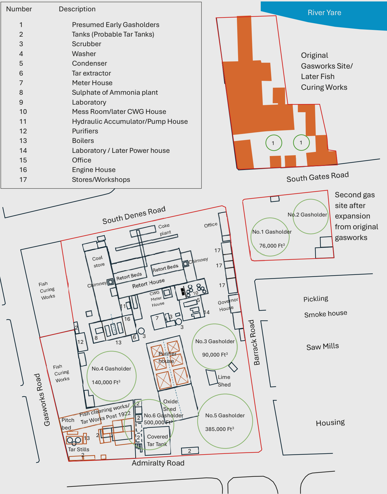
Figure 30. A plan of how the Great Yarmouth Gasworks developed, showing the principal features. Source: Russell Thomas.
