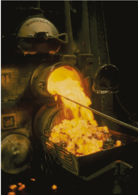
Figure 50. Removing hot coke from the retorts. Source: National Gas Archive.
