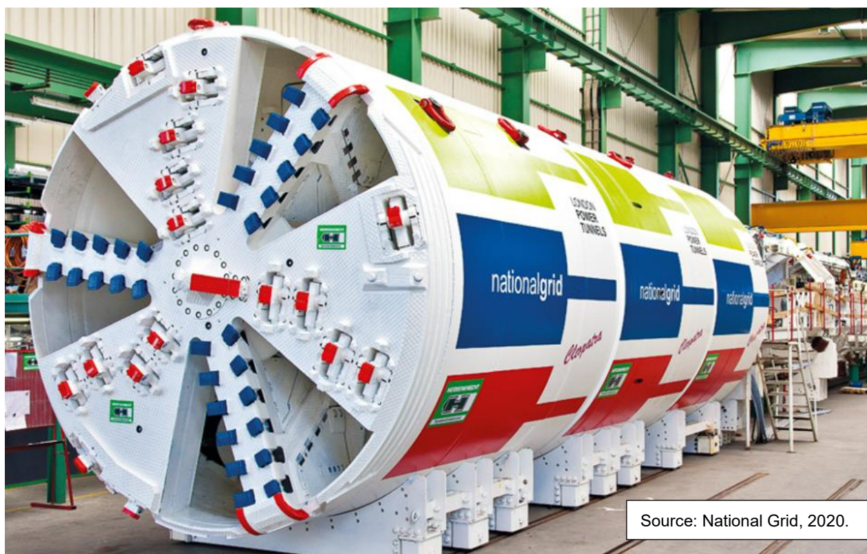
Figure 3-7: Example Tunnel Boring Machine
