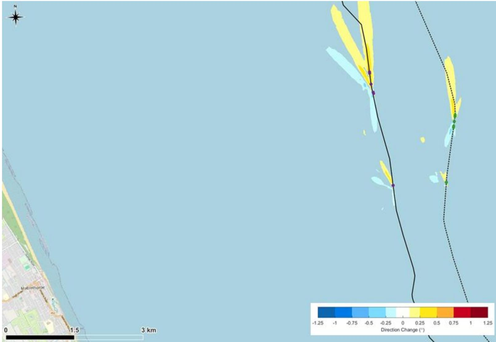
Figure 15. Predicted change in wave direction during a large wave from the southeast due to the rock berms at the 12 crossings.
