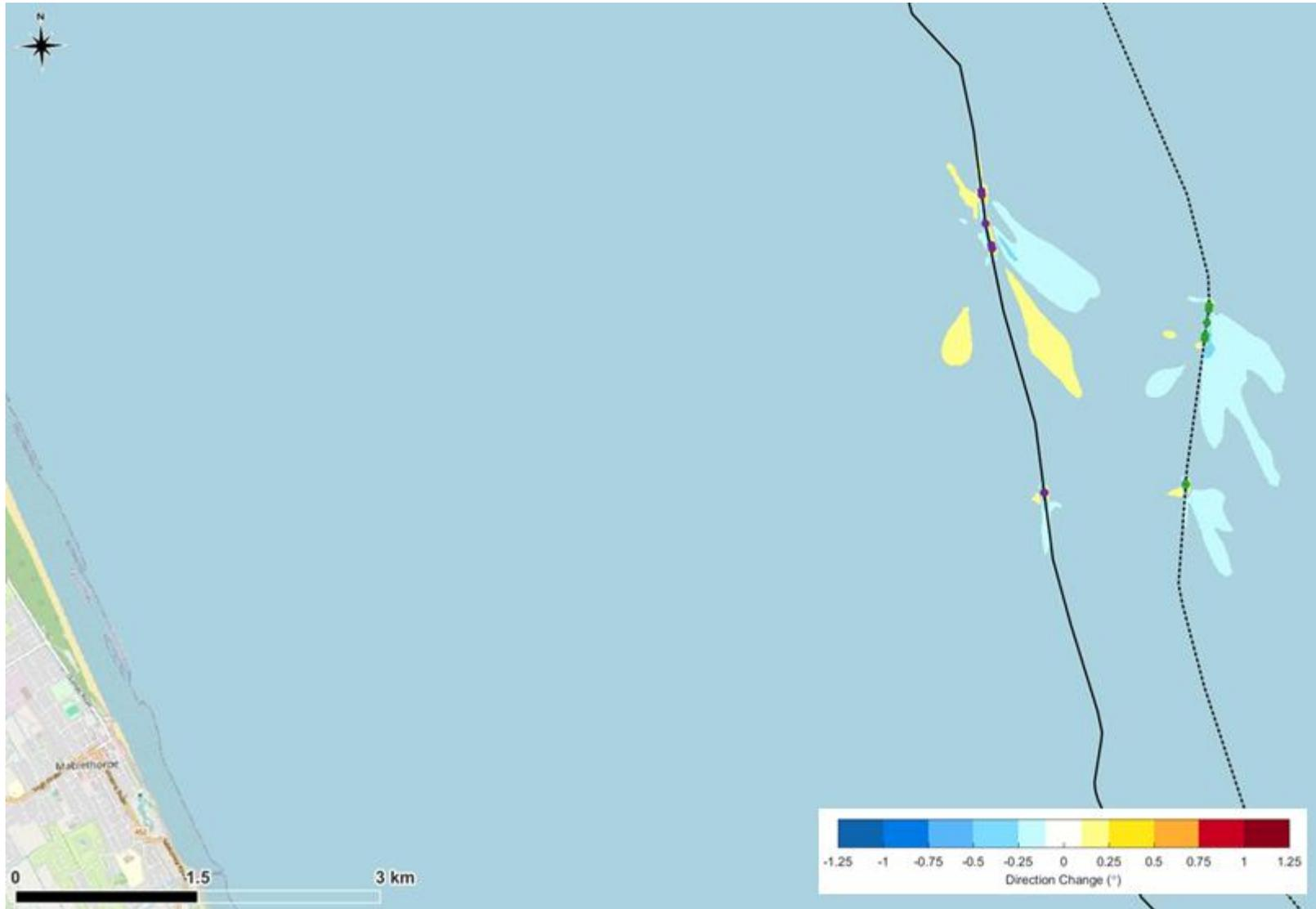
Figure 12. Predicted change in wave direction during a large wave from the north due to the rock berms at the 12 crossings.
