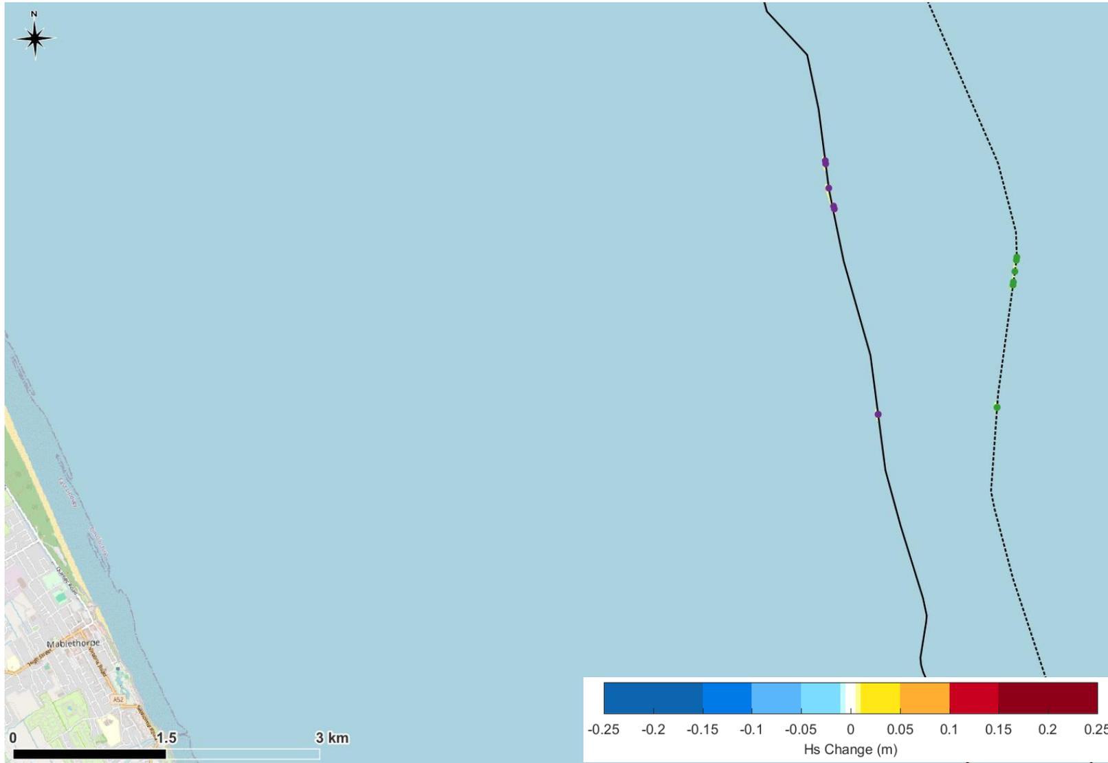
**Figure 11.** Predicted change in  $H_s$  during a large wave from the south due to the rock berms at the 12 crossings.
