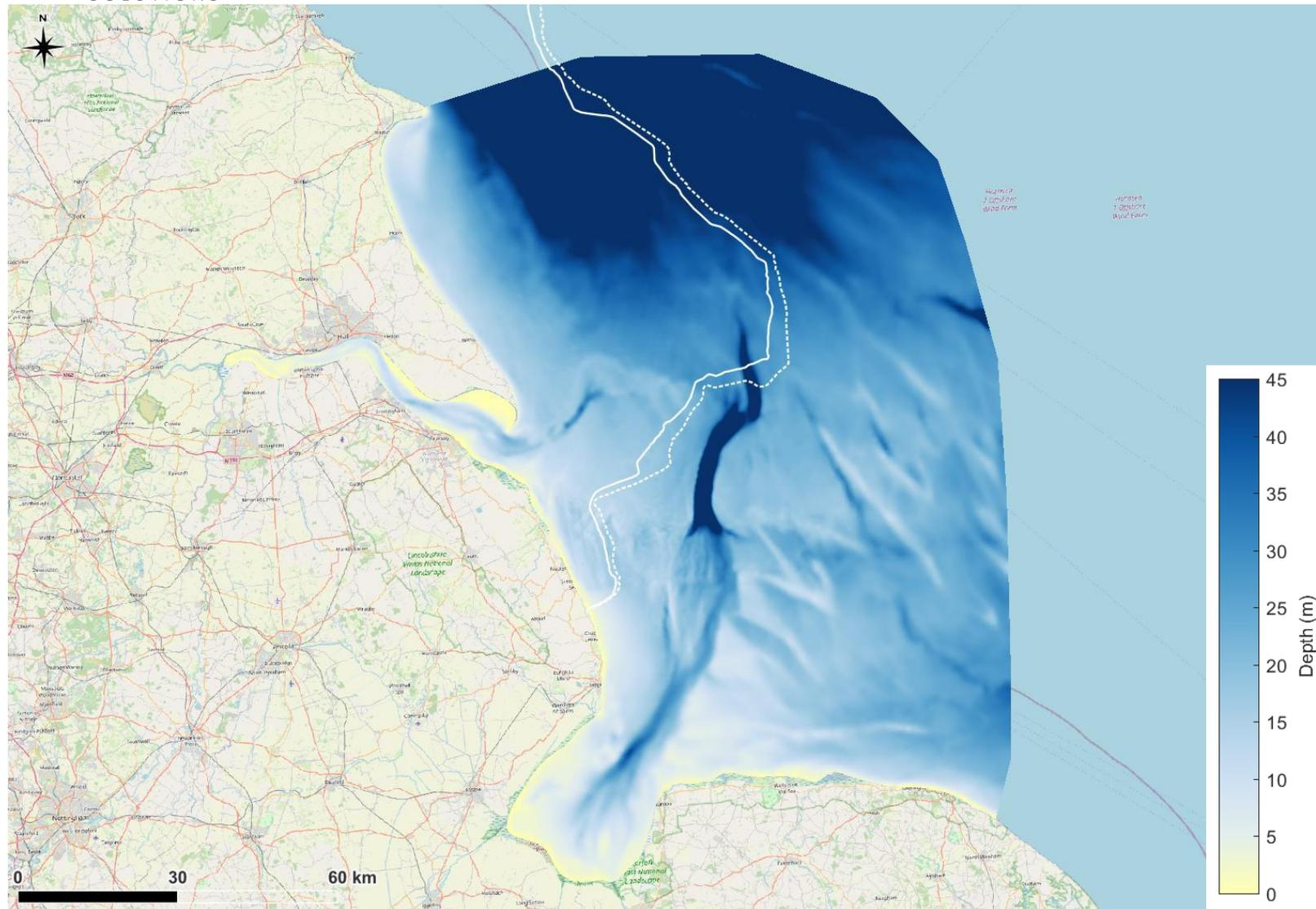
**Figure 5. Model bathymetry along with the EGL 3 and EGL 4 cable routes.**
