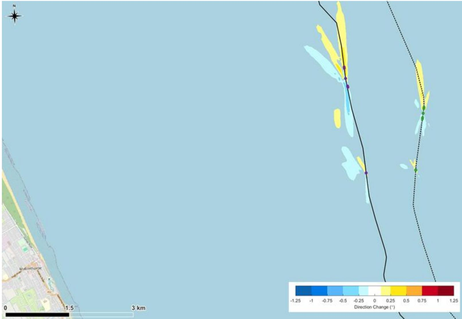
**Figure 14.** Predicted change in wave direction during a large wave from the east due to the rock berms at the 12 crossings.
