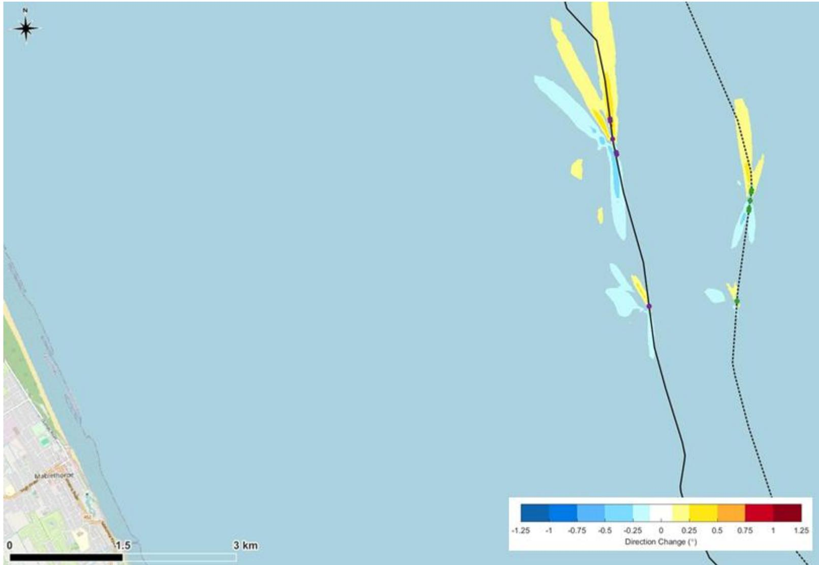
Figure 16. Predicted change in wave direction during a large wave from the south due to the rock berms at the 12 crossings.
