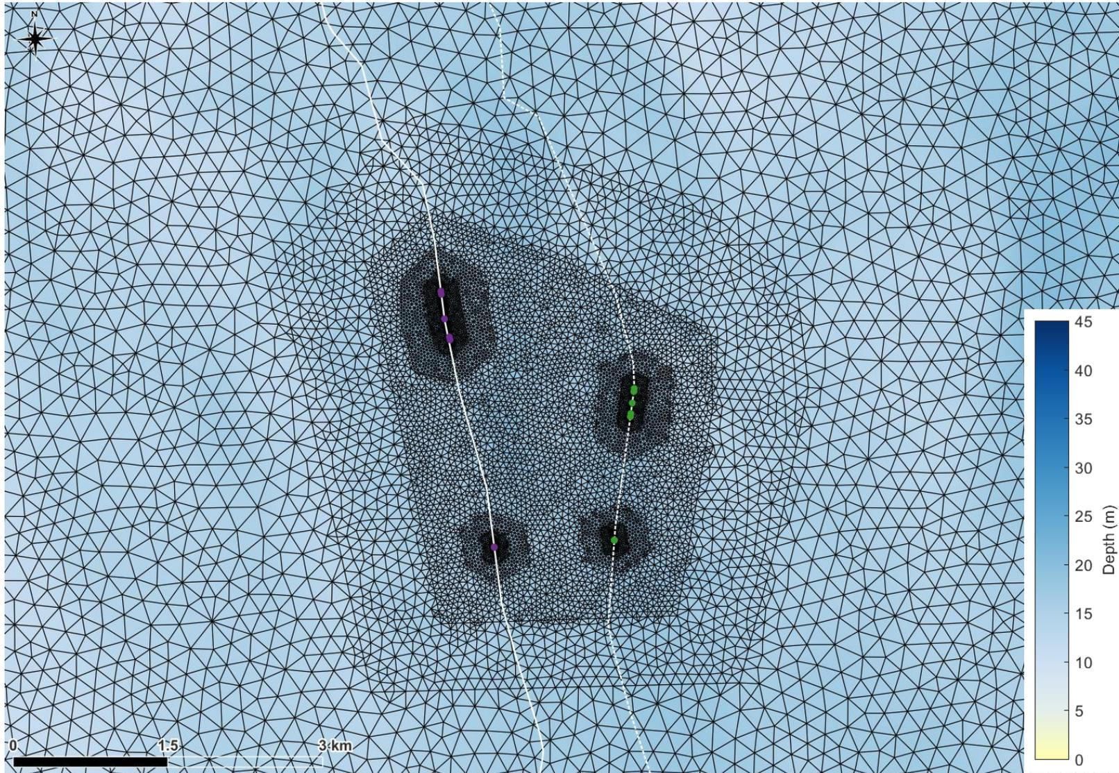
Figure 4. Close up of the SW model mesh and bathymetry at the crossing locations (purple dots = EGL 4 crossings; green dots = EGL 3 crossings).
