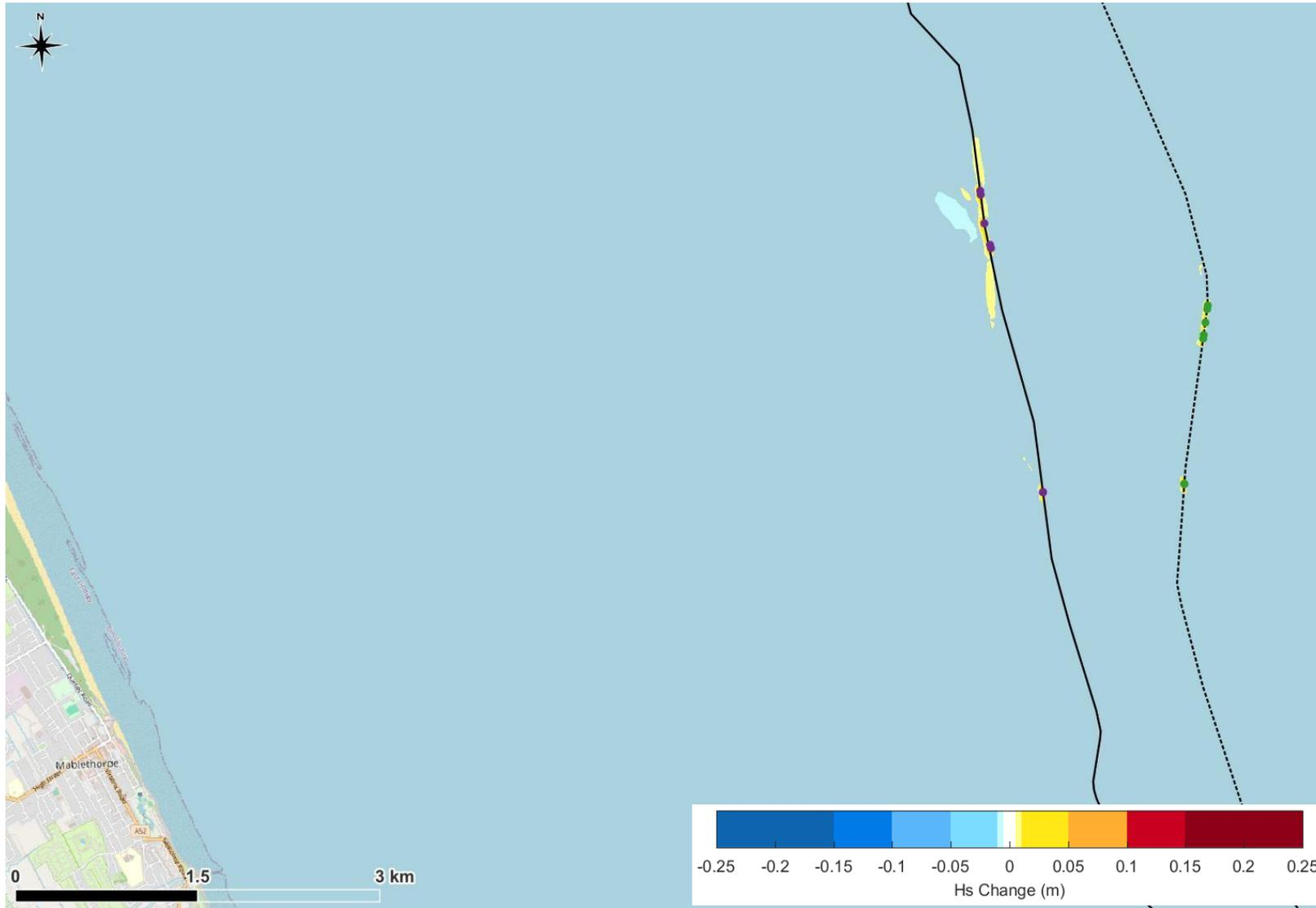
**Figure 9.** Predicted change in  $H_s$  during a large wave from the east due to the rock berms at the 12 crossings.
