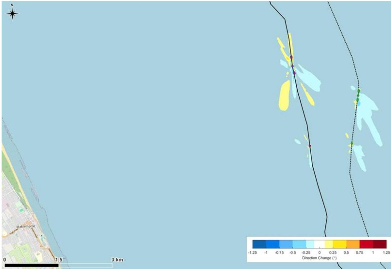
Figure 13. Predicted change in wave direction during a large wave from the northeast due to the rock berms at the 12 crossings.
