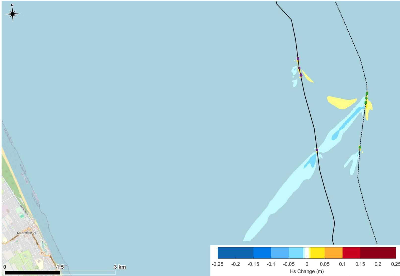
**Figure 7.** Predicted change in  $H_s$  during a large wave from the north due to the rock berms at the 12 crossings.
