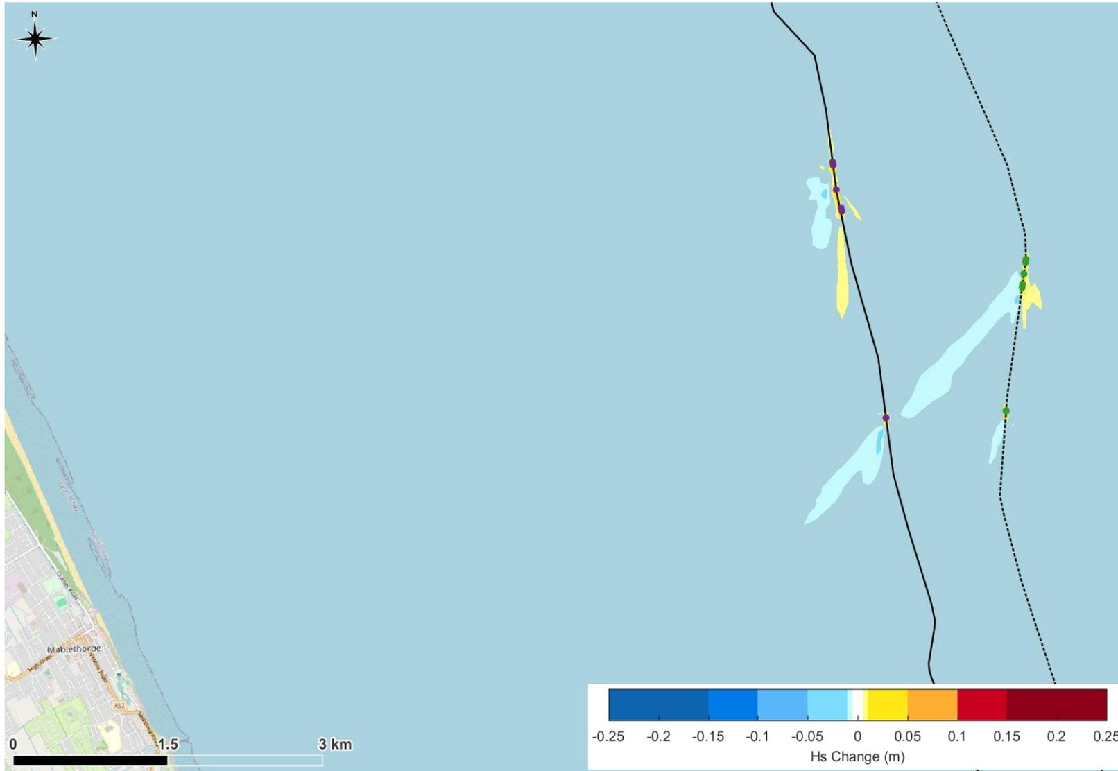
**Figure 8.** Predicted change in  $H_s$  during a large wave from the northeast due to the rock berms at the 12 crossings.
