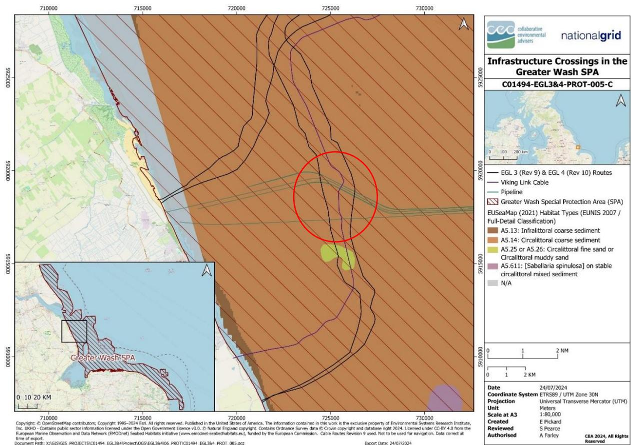
**Figure 2.** Location of EGL 3 and EGL 4 cable and pipeline crossings close to the landfall (CEA, 2024).
