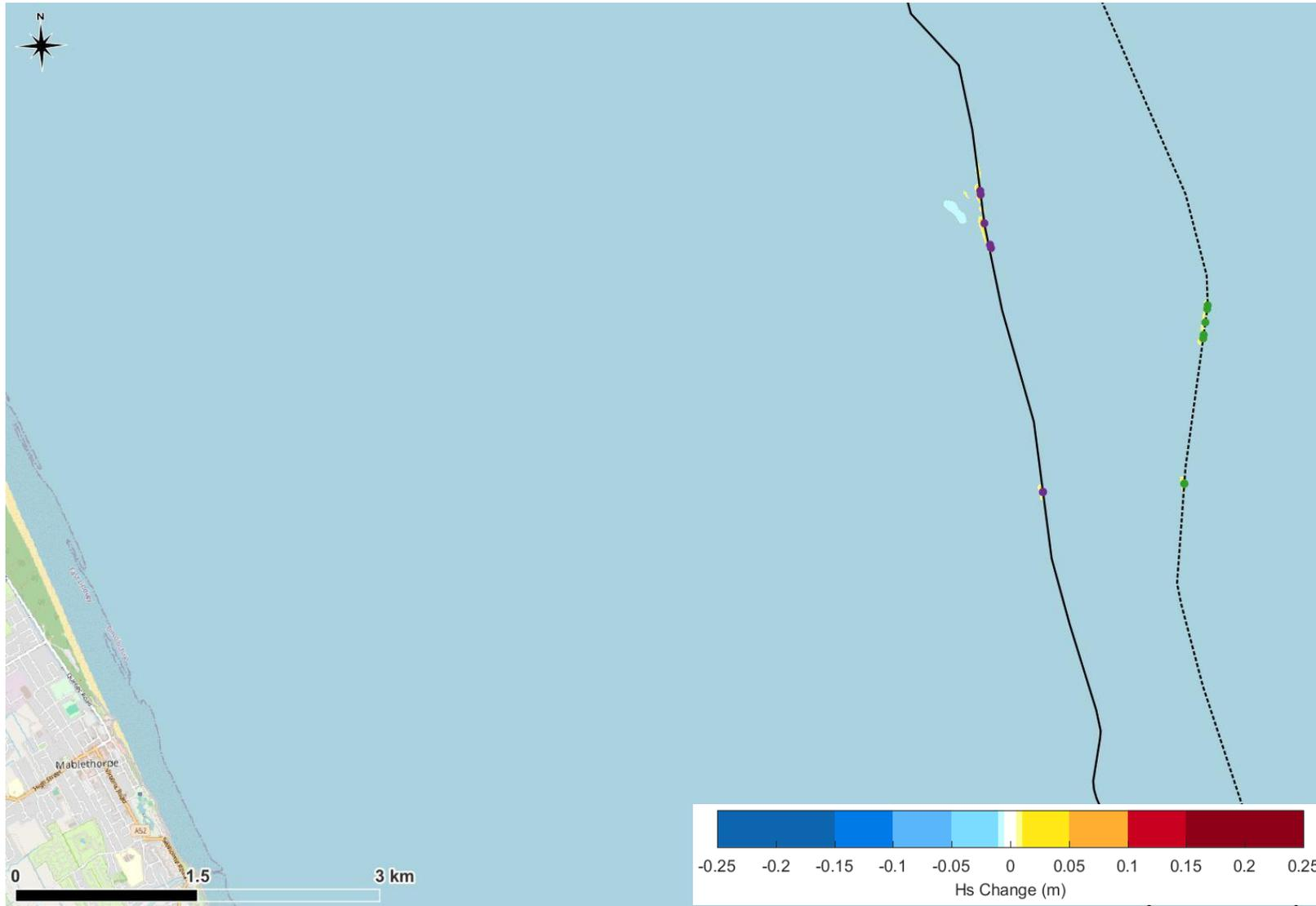
**Figure 10.** Predicted change in  $H_s$  during a large wave from the southeast due to the rock berms at the 12 crossings.
