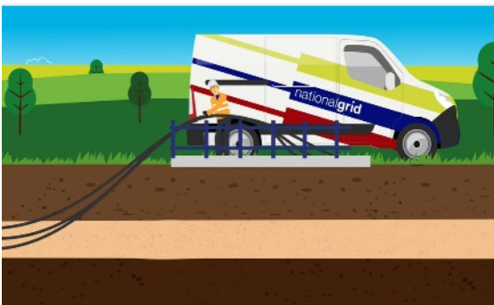
Step 5 The cables are then laid along the length of the trench within ducts
