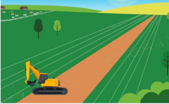
Step 1 Cables are installed in two (HVDC) or four (HVAC) trenches, adjacent to the temporary haul route
