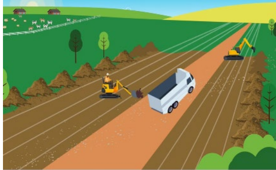
Step 2 The topsoil is carefully removed and stored separately alongside the trenches so it can be put back after the work is complete
