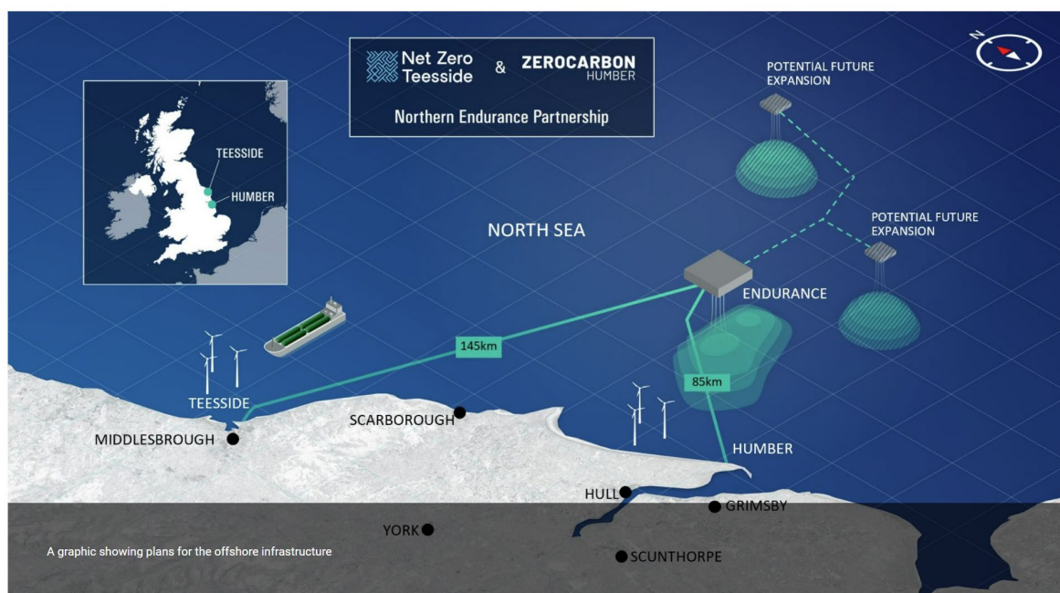
Figure C-8: Diagram showing the offshore infrastructure at Teesside and Humber. Taken from BP, (2023)
