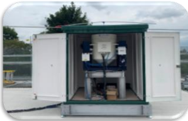
500 kN shaker for mechanical testing
