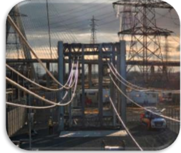
20 and 90 m spans conductor test rigs
