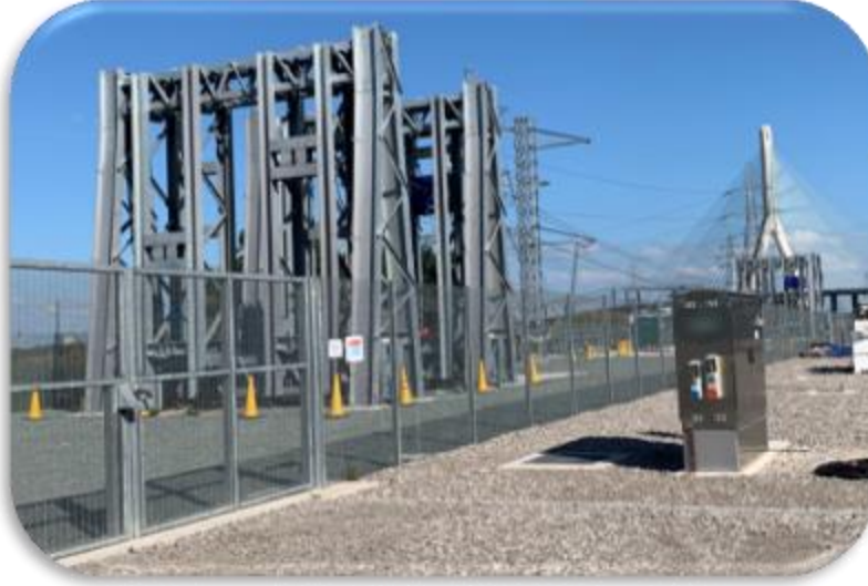
20 and 90 m spans conductor test rigs
