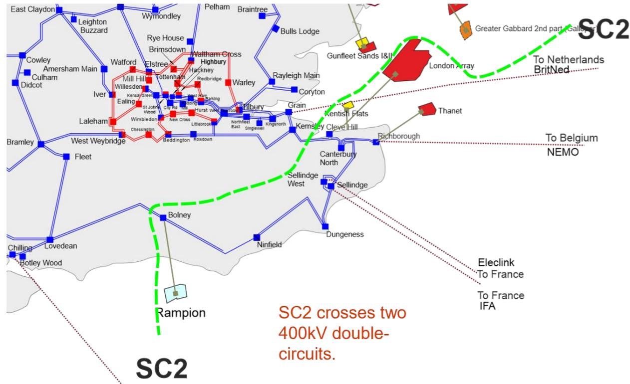
The relatively long 400kV route between Kemsley and Lovedean feeds significant demand and connects both large generators and interconnection to Europe. A fault at either end of the route can cause it to become a long radial feeder which puts all loading on the remaining two circuits which can be restrictive due to circuit ratings and cause voltage issues.
