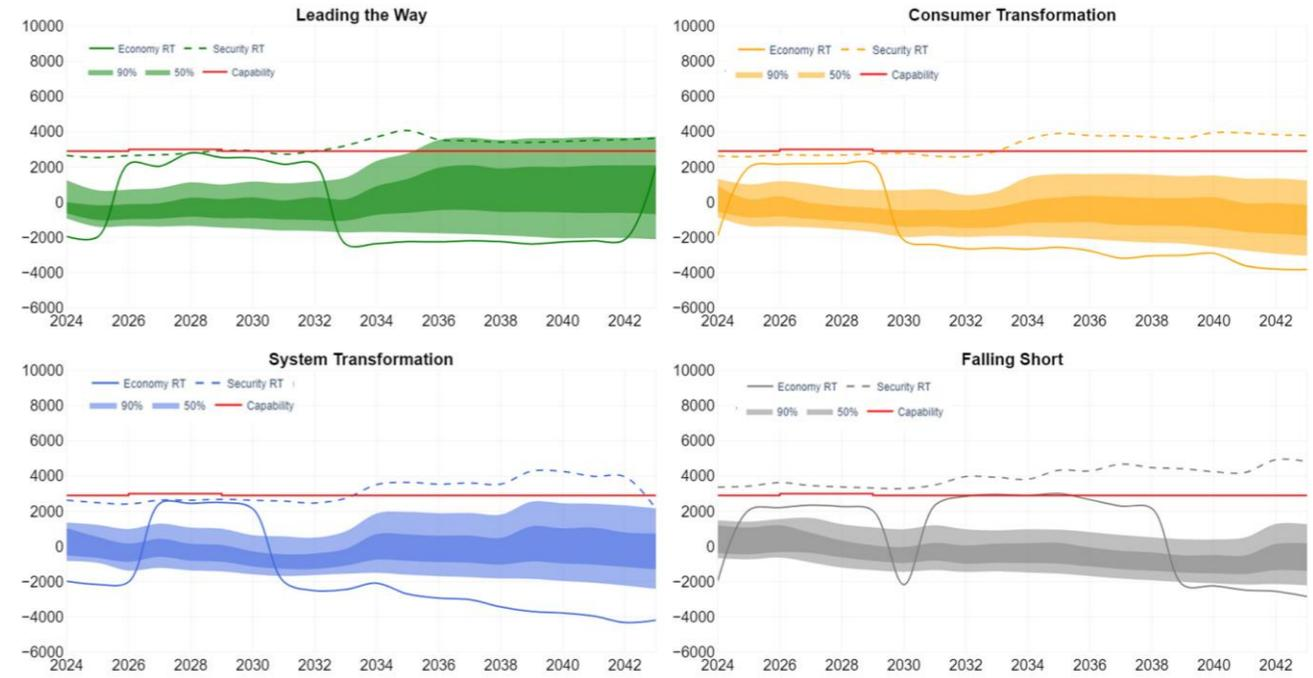
The capability line (in red) is based on the recommendations from the NOA Refresh 2021/22 optimal path which uses the 2021 FES and ETYS data as inputs. The 50%, 90%, Economy RT and Security RT lines are based on FES 2023. The ETYS and NOA methodologies for this boundary are different and can result in different transfer capabilities.
