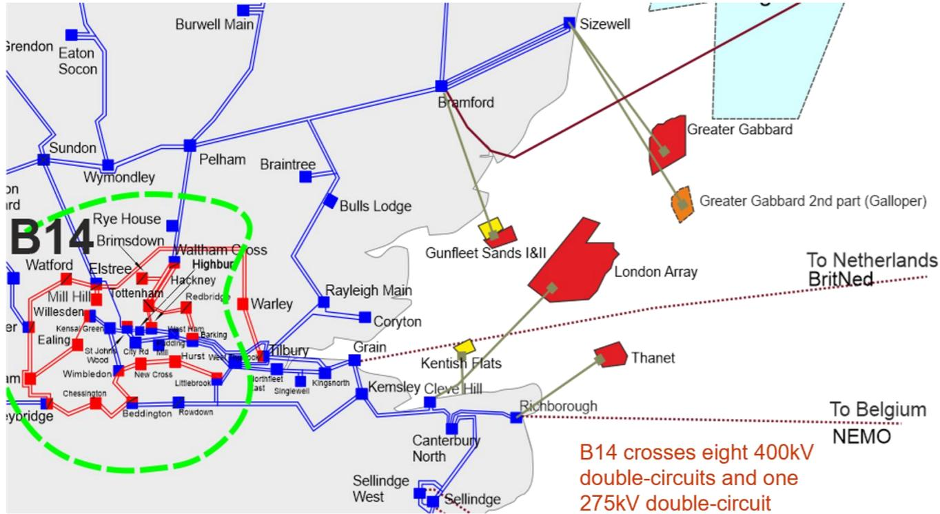
The circuits entering from the north can be particularly heavily loaded at winter peak conditions. The circuits are further overloaded when the European interconnectors export to mainland Europe as power is transported via London to feed the interconnectors along the south coast.
