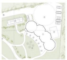
The primary elevation of the 4 tipis will face to the south west into the site and have the facility to be opened up onto a hard surface patio area to provide additional seating. This will be designed to be free draining as part of the site wide drainage strategy.
