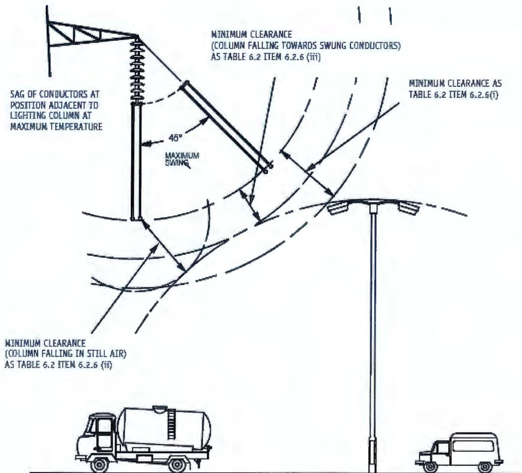
Fig. 3 HV Conductor Clearance to lighting columns
