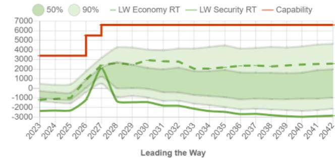
It can be seen that until new generation or interconnectors connect there is very little variation in boundary requirements, and that the current importing boundary capability is sufficient to meet the short-term needs.
