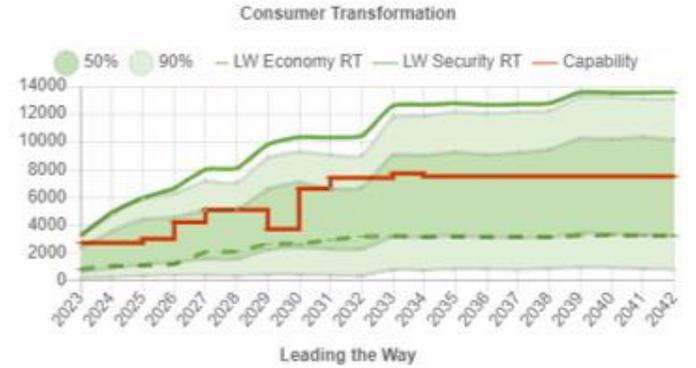
The capability line (in red) is based on the recommendations from the NOA 2021/22 optimal path which uses the 2021 FES and ETYS data as inputs. The 50%, 90% Economy RT and Security RT lines are based on FES 2022. The ETYS and NOA methodologies for this boundary are different and can result in different transfer capabilities.
