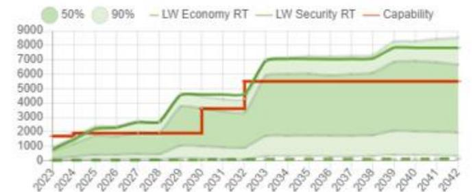
The power transfer through B0 is increasing due to the substantial growth of renewable generation north of the boundary. This generation is primarily centred around both onshore and offshore wind. There is also the prospect of new marine generation resource in the Pentland Firth and Orkney waters in the longer term.
