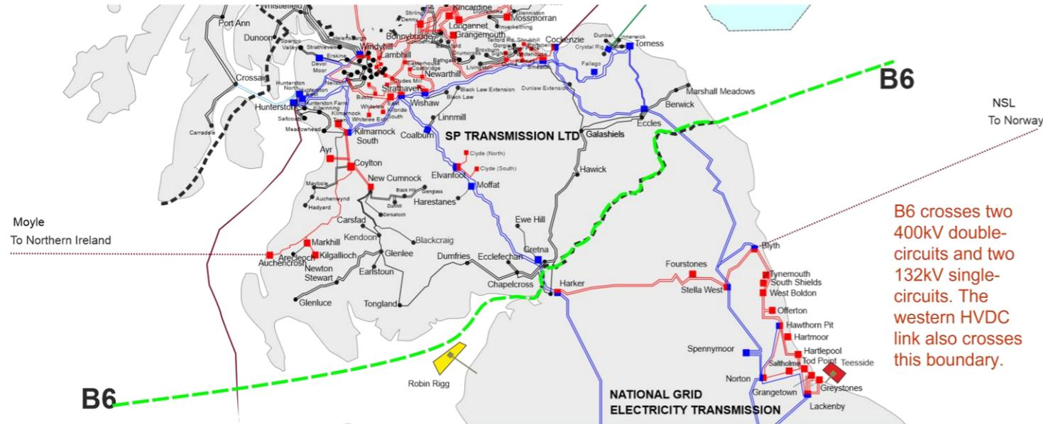
B6 crosses two 400kV double-circuits and two 132kV single-circuits. The western HVDC link also crosses this boundary.
