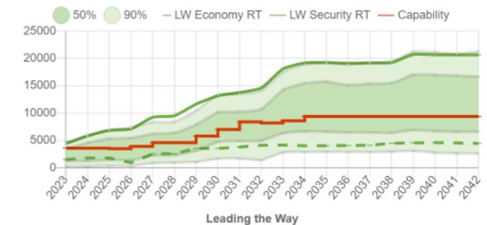
The capability line (in red) is based on the recommendations from the NOA 2021/22 optimal path which uses the 2021 FES and ETYS data as inputs. The 50%, 90% Economy RT and Security RT lines are based on FES 2022. The ETYS and NOA methodologies for this boundary are different and can result in different transfer capabilities.
