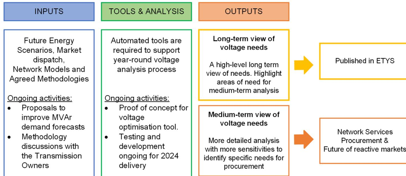
**Inputs:** The voltage analysis process will take generation and demand profiles from the FES scenarios which will be fed into our market dispatch tool to produce a credible year-round economic dispatch that is applied to our network models. We are in the process of reviewing the methodology with the Transmission Owners and we are progressing actions to improve our MVAR demand forecasts.
