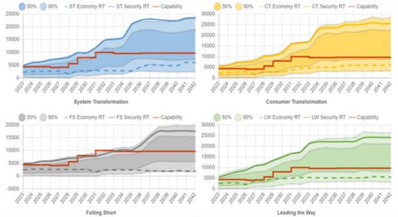
The capability line (in red) is based on the recommendations from the NOA 2021/22 optimal path which uses the 2021 FES and ETYS data as inputs. The 50%, 90% Economy RT and Security RT lines are based on FES 2022. The ETYS and NOA methodologies for this boundary are different and can result in different transfer capabilities.
