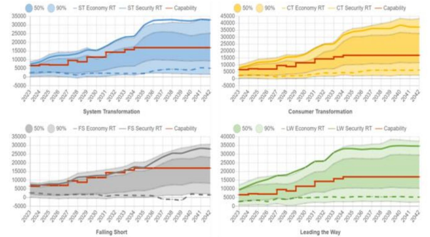
Across all FES, there is an increase in the power transfer requirements from Scotland to England due to the connection of additional generation in Scotland, primarily onshore and offshore wind.
