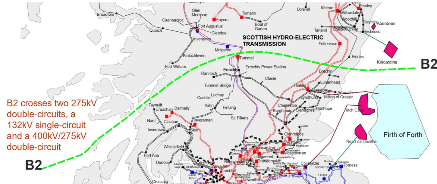
The potential future boundary transfers for boundary B2 are increasing at a significant rate because of the high volume of renewable generation to be connected to the north of the boundary. This increased generation capacity will drive increasing power flows down the east coast 275kV circuits.
