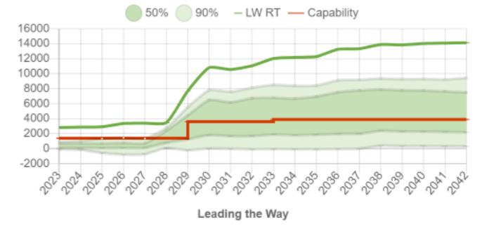
Currently, there is not a significant amount of generation behind NW2, mainly Dinorwig pumped storage and offshore wind projects connecting to Bodelwyddan. The expected transfers only see significant changes from around 2029 onward when they increase very sharply as large new offshore wind projects come online and an intra GB DC link connecting to Scotland lands at Pentir. This will mean that in future transfers across the NW2 boundary will be heavily dependent on wind conditions.
