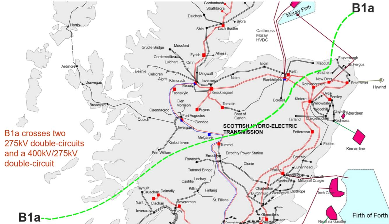
New renewable generation connections north of the boundary are expected to result in a significant increase in export requirements across the boundary, especially along the Beaulay – Denny circuit. All generation north of boundary B0 also lies behind boundary B1a.
