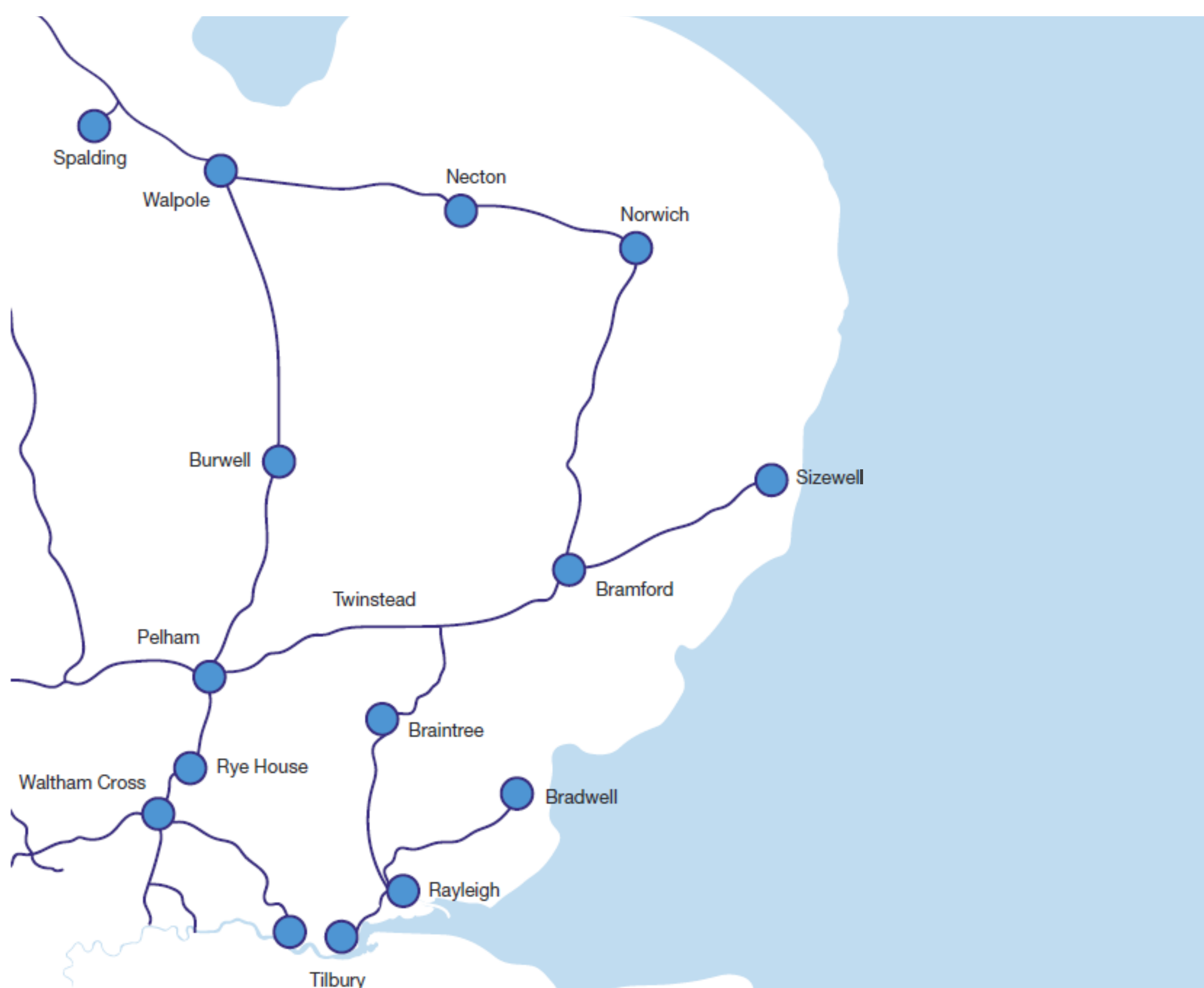
Figure 1 The existing high voltage transmission network in East Anglia
