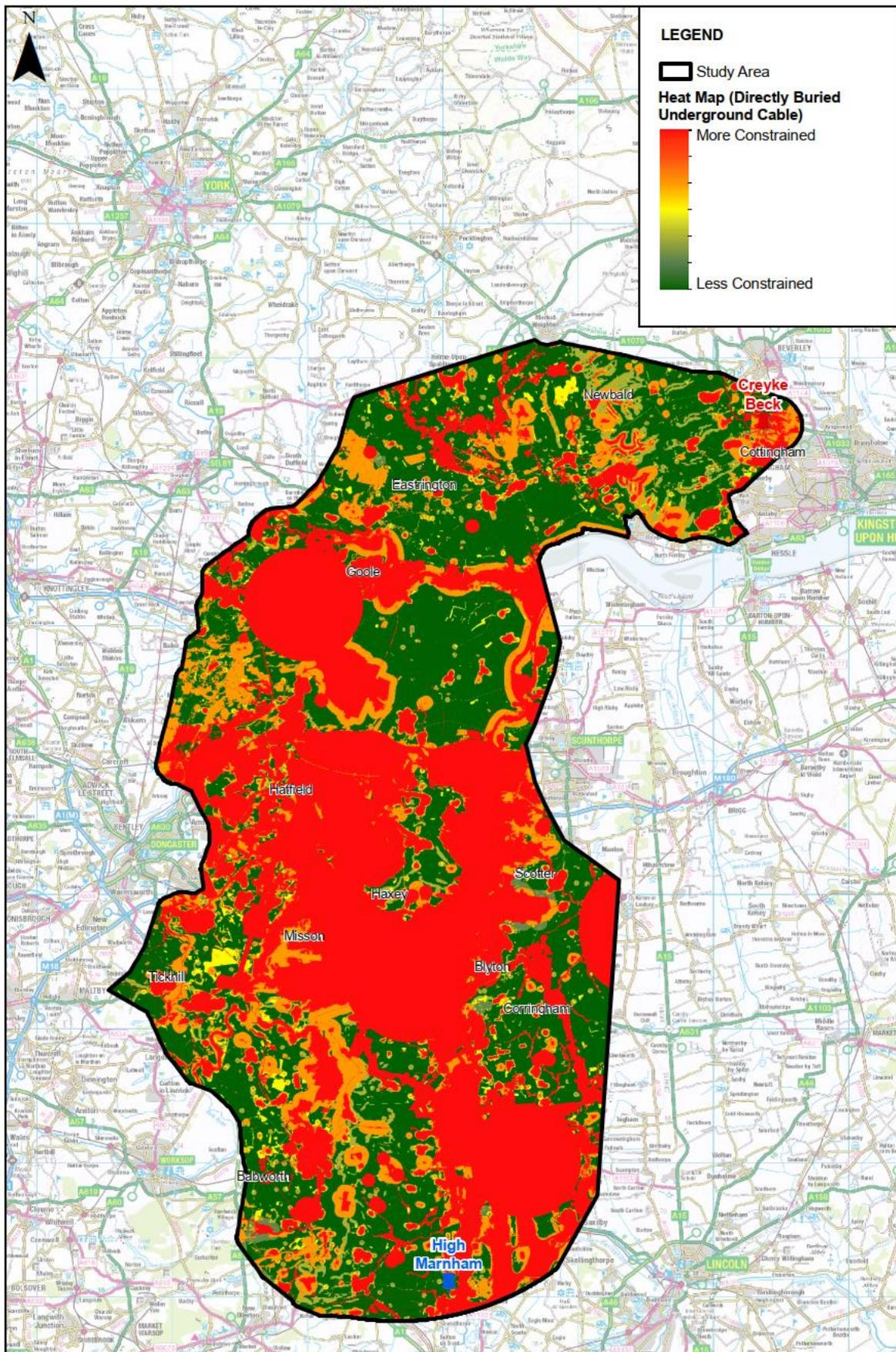
Figure 5-7 – Heat Map (Directly Buried Underground Cable)
