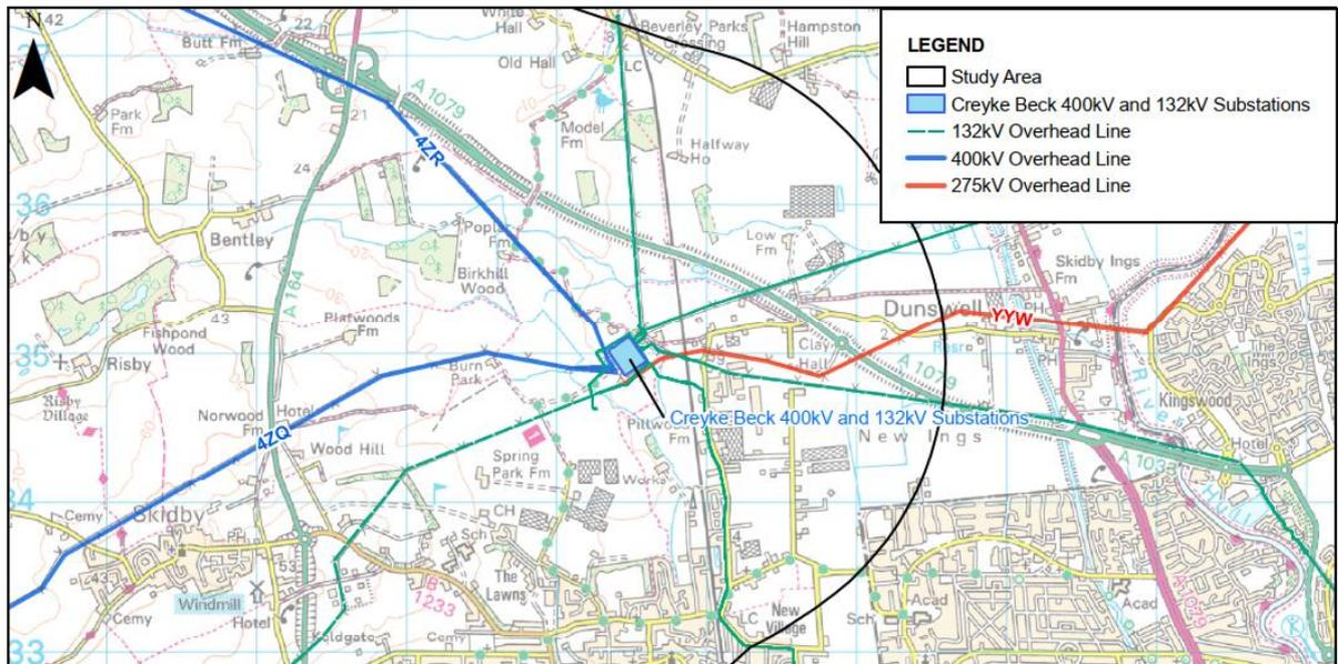
Figure 2-8 – Location of the Existing 400kV Creyke Beck Substation, Adjacent 132kV Substation and Connecting Overhead Lines
