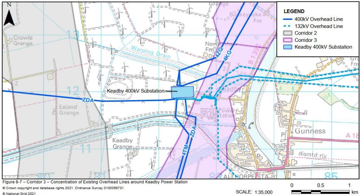
Figure 8-7 – Corridor 3 – Concentration of Existing Overhead Lines around Keadby Power Station
