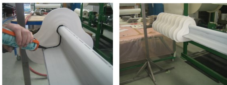
Sheds are slid down over the horizontal profile and sealed with silicone
