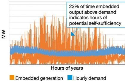
The graph above shows that the wind and solar output (embedded generation) alone is insufficient to meet hourly demand 78% of the time (i.e. when the orange trace is below the blue trace), with the worst shortfall reaching 3 GW.
