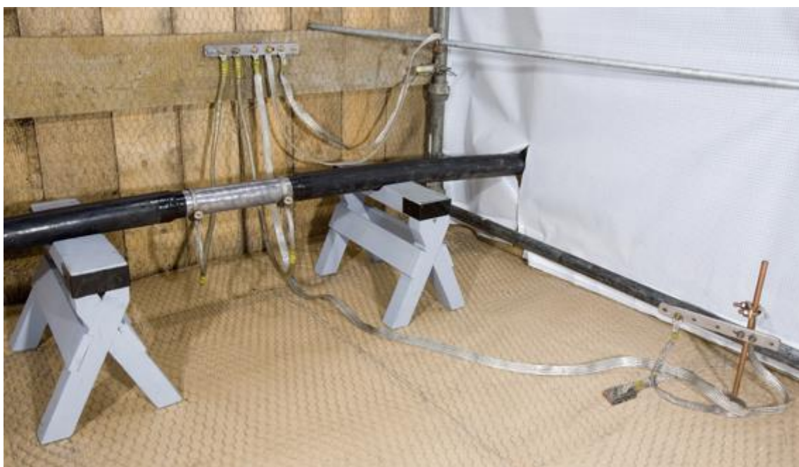
A photograph of a bay set for Earthed Working .
