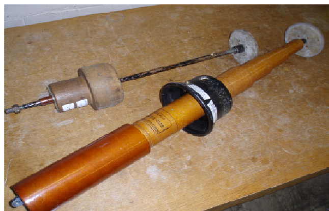
Figure 5.4B – Test Bushings for Metal Clad Switchgear
