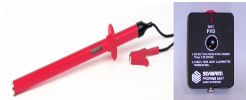
Figure 4.1A - Potential Indicator (SEAWARD KD1E/33) and Proving Unit
