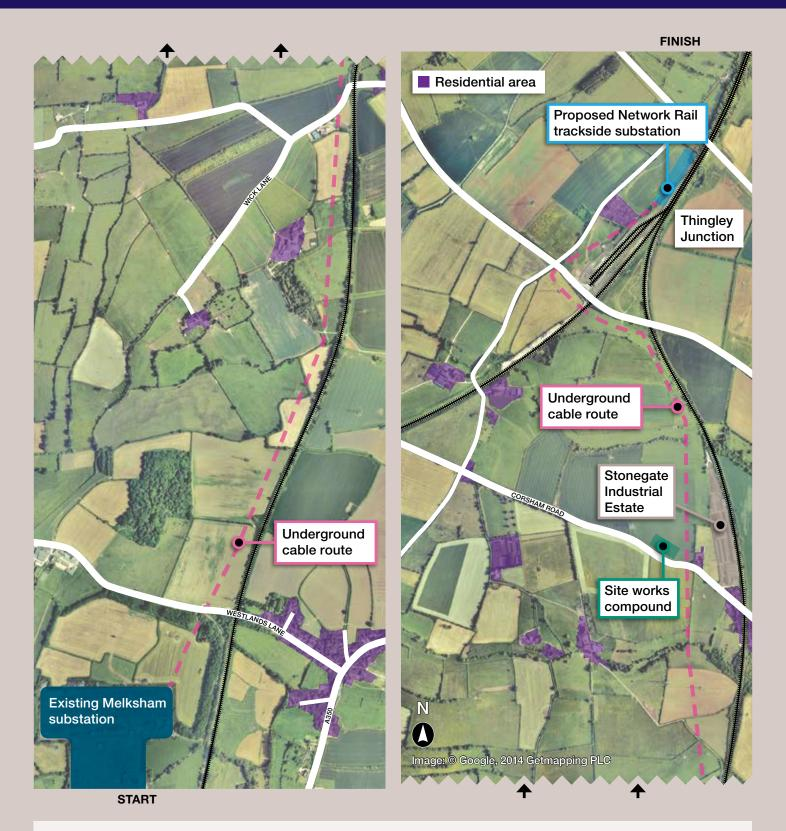
This map, split into two sections, shows the route National Grid will take when installing new underground cables from its existing Melksham substation to a new trackside substation near Thingley Junction. This is part of our work with Network Rail to electrify the Great Western Main Line railway. The route goes north, broadly following the rail-line, going underneath Westlands Lane, Wick Lane, Corsham Road and the road near Thingley Junction.
