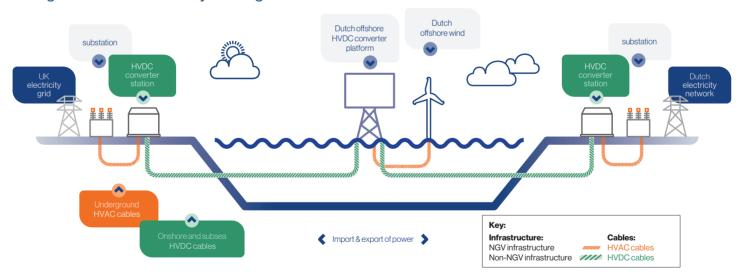
**Undersea and underground:** a key feature of the project is that no cables will be seen in the local area at all: they are all subsea or underground.
