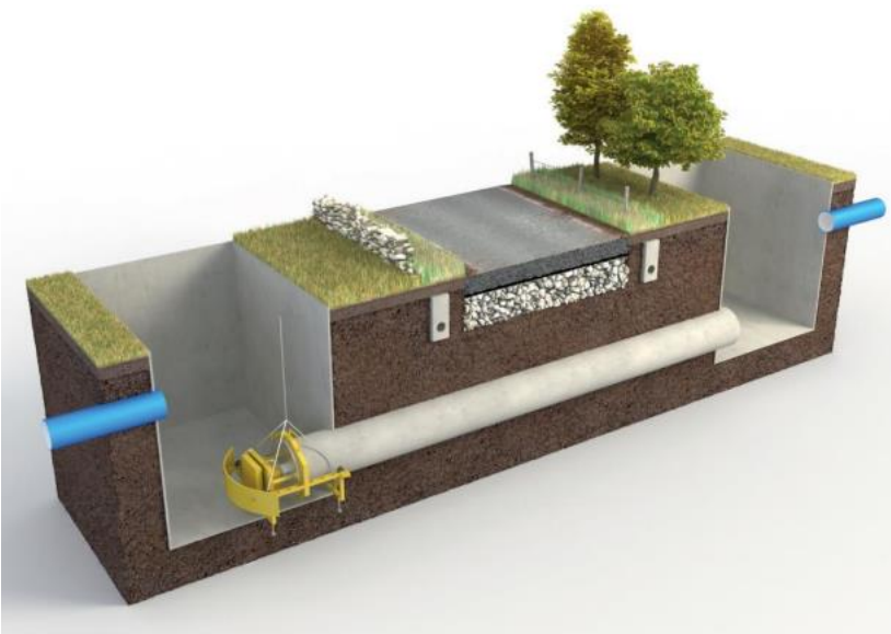
Insert 2.4: Illustration of Micro-tunnelling technique (Ref 2.3).
