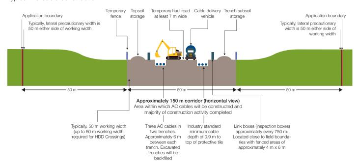
This illustration is for illustrative purposes only and is intended to show the typical construction of AC cables for interconnectors in the UK
