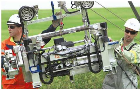
A remotely operated overhead lines inspection and maintenance robot will make it easier and safer to maintain the high voltage overhead line network in the UK.
