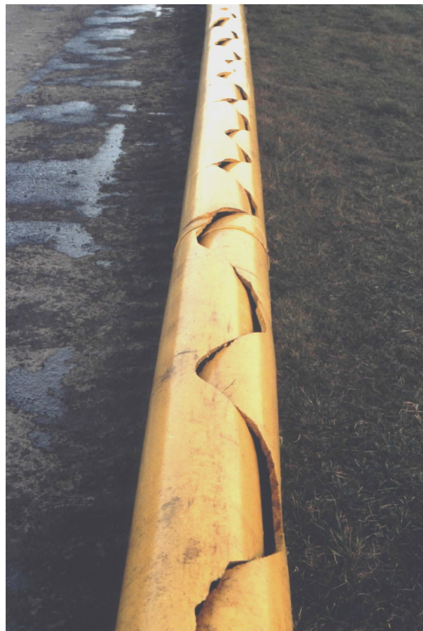
Figure G.1 RCP in 315 mm SDR 17.6 PE80 pipe
